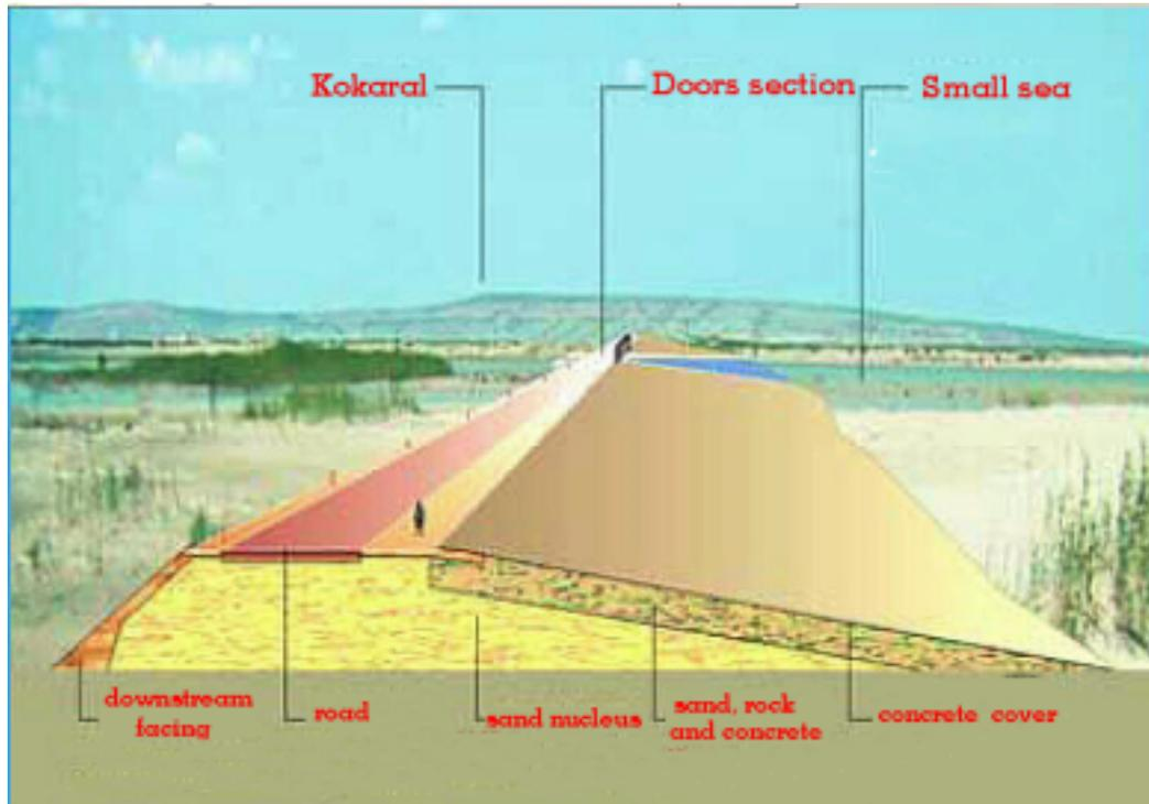
Schematic view of the dyke structure
