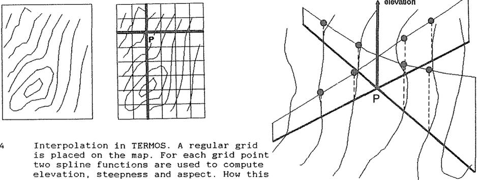
FIG. 4 Interpolation in TERMOs. A regular grid is placed on the map. For each grid point two spline functions are used to compute elevation, steepness and aspect. How this is done for grid point P is shown to the right.
