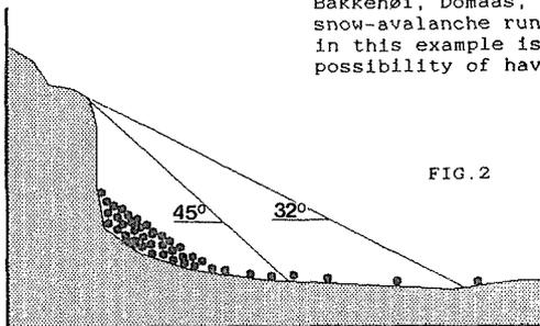
FIG.2 Run-out distance for 50% ( $45^\circ$  line) and 95% ( $32^\circ$  line) of the rocks falling from the cliff.
