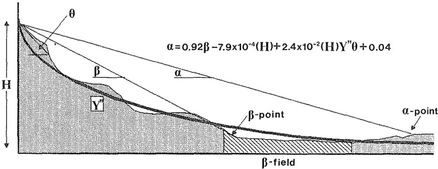
FIG.1 Formula and topographical parameters used in the Bakkehøi, Domaas, Lied method for computation of snow-avalanche run-out distance. The topography in this example is exaggerated to exemplify the possibility of having several potential  $\beta$ -points.
