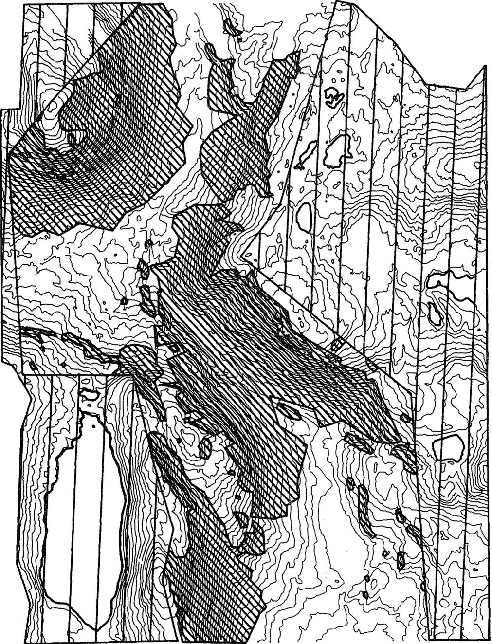
FIG. 7 The final map, ready for printing. All the map examples are made using a small section (40 km<sup>2</sup>, scale 1:39.667) from a M711 map. Ordinary survey mapping is performed on the entire map (400 to 600 km<sup>2</sup>, scale 1:50.000). The avalanche zones are filled in with colour on the finished map, and not hatched as in this example.
