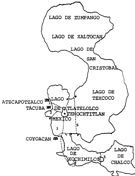
FIG.2 Major flood control works at Mexico-Tenochtitlan. (1) Tlatelolco-Atzacapotzalco road, (2) Tacuba road, (3) Coyoacan-Xochimilco road, (4) Mexicalzingo road, (5) Cuitlahuac road, (6) Netzahualcoyotl's dike, (7) Tepeyac road.
