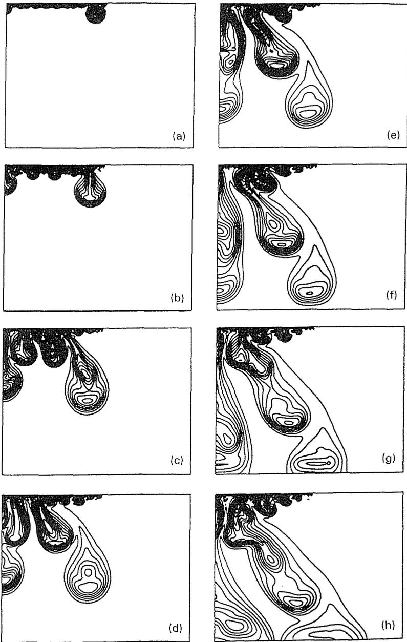
Fig. 2 Developmental stages of unstable plumes in Hele-Shaw cell using the SUTRA solute transport model. Elapsed times (a,b,...,h) given in dimensionless times are  $T = 2.01, 4.02, 8.03, 10.05, 12.06, 14.06, 16.07, 18.08$ , measured from start of numerical simulation.
