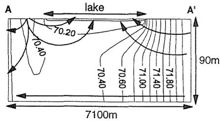
Fig. 8 Modelled hydraulic head (in m) for January 1994.
