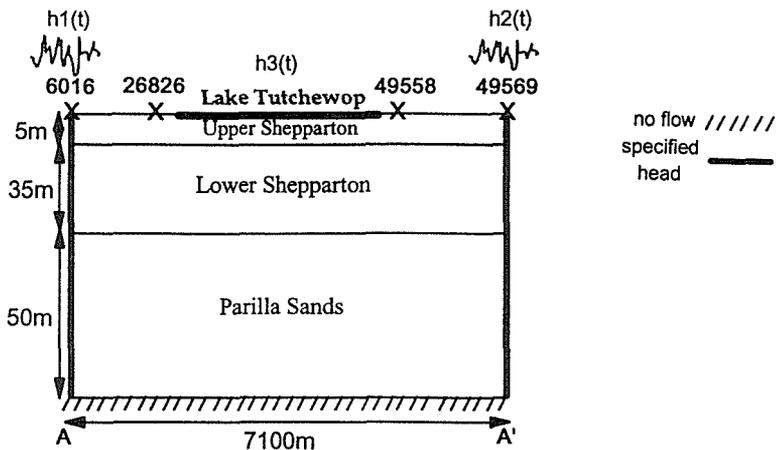
Fig. 3 2D cross-sectional view of Lake Tutchewop model, with boundary conditions.
