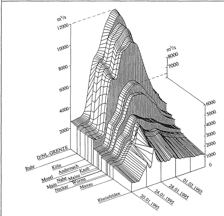
Fig. 3 Stereographic representation of the flood waves of December 1993/January 1994 and January 1995 on the River Rhine.
